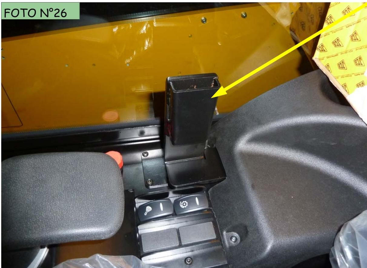
VISTA SUPPORTO Cod. **DM600180** LEVA FRENO RIMORCHIO DA MONTARE IN CABINA ALLA " DX " SEDILE DI GUIDA, FISSARE CON N°4 VITI TE M8x25 + DADO AUT .
